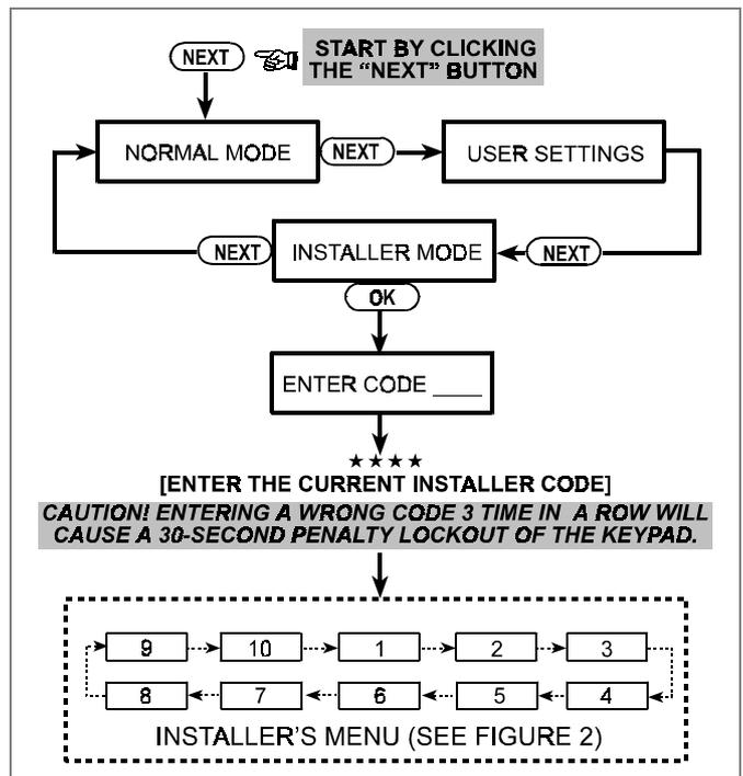
Figure 1. Gaining Access to the Installer's Menu
