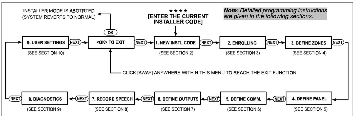
Figure 2. Navigating within the Installer Menu
